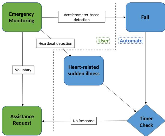
Fig. 3: Representation of unconsciousness detection model. In Green the processes that are embedded in the wearable system and depend from the user interaction, in Blue the logic that runs on the smartphone (timer check) or the Fog node
