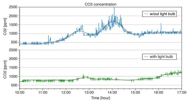
Fig. 2: Trends of CO<sub>2</sub> concentration before (top) and after (bottom) the installation of the light bulb inside the laboratory room. In the *before* graph are visible the curves caused by meetings during the day.
