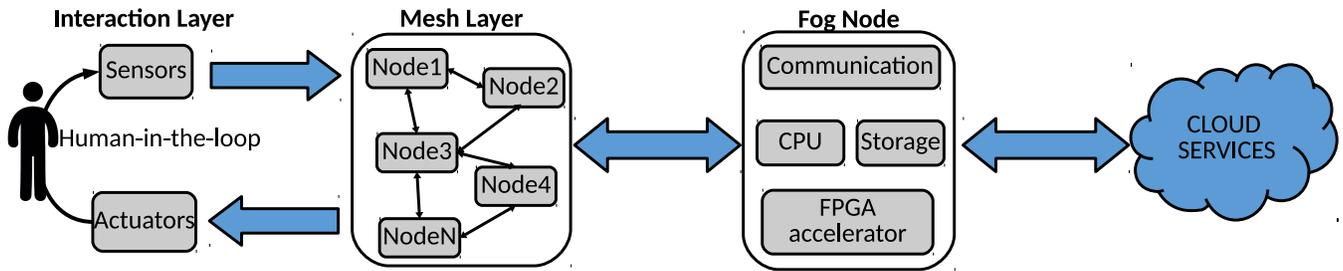
Fig. 1: Representation of the proposed architecture. The Interaction Layer collect data and receive commands. The Mesh Layer aggregate data, transfer commands and handle the security of lower nodes. The Fog Node process data to act on the ambient and possibly transfer information to the Cloud.
